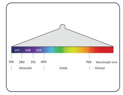
UV-C lamps used in UV-C Disinfection system, have their main emission at 254 nm where the action on DNA is 85% of the peak value and 80% on the IES curve. As a result, our germicidal lamps are extremely effective in breaking down the DNA of micro-organisms. This means that they cannot replicate and cause disease.
